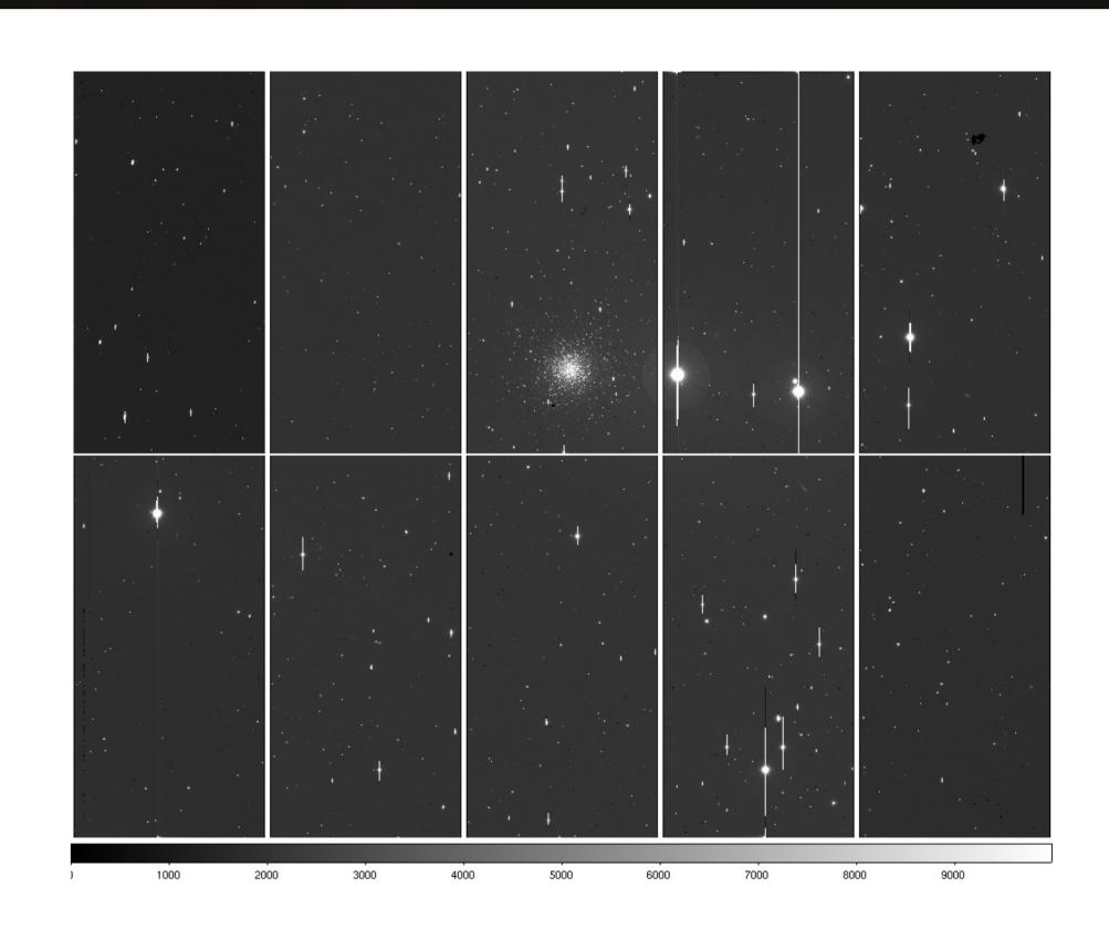
A SuprimeCam exposure (V filter, 180 s) in the field of NGC 2419. The cluster is located in the upperrow, central chip. SuprimeCam is a 10-chip (2K×4K) mosaic camera at the prime focus of the Subaru 8-m telescope at Mauna Kea, Hawaii. Pixel scale is 0.2" and field of view is 34'×27'.
