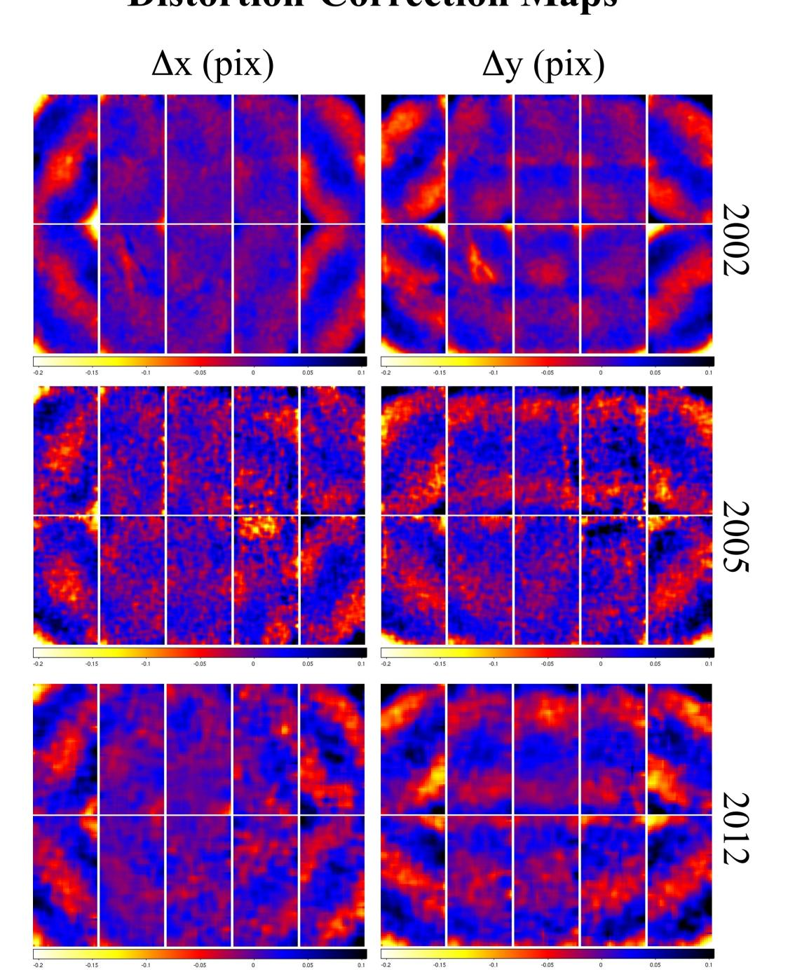
The derived astrometric correction maps, by epoch, of distortions beyond cubic field terms.
